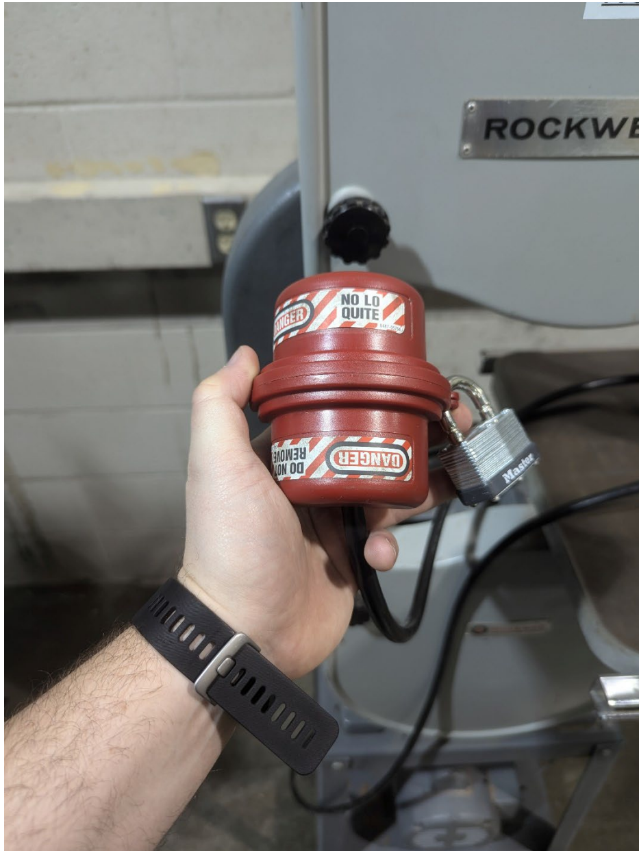
Figure 1 A lock ensures only trained operators may use the equipment.
