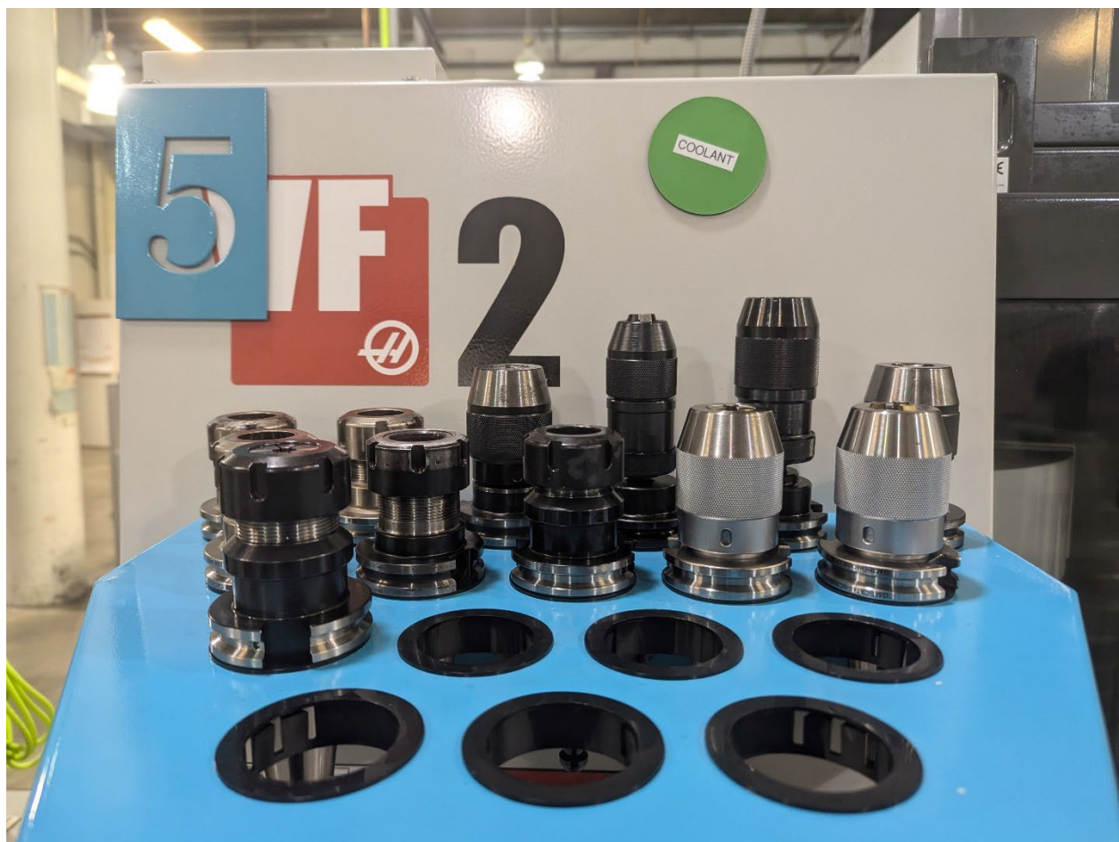
Figure 2 CNC Machines have color-coded tools that should be kept with each machine.
